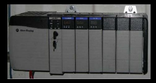
Allen-Bradley 1756 Control Logix / Compact Logix Processor to Interface with existing Allen-Bradley Type PLC Controls and Infilink HMI Software. (DH+, Remote I/O, & Ethernet Comms)
